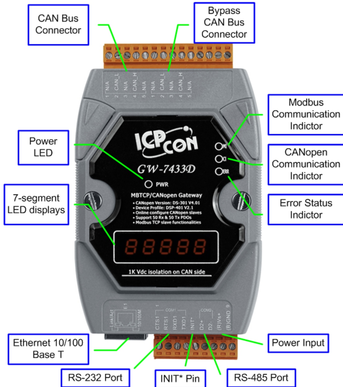
Figure 2.1 Pin assignments on the GW-7433D
