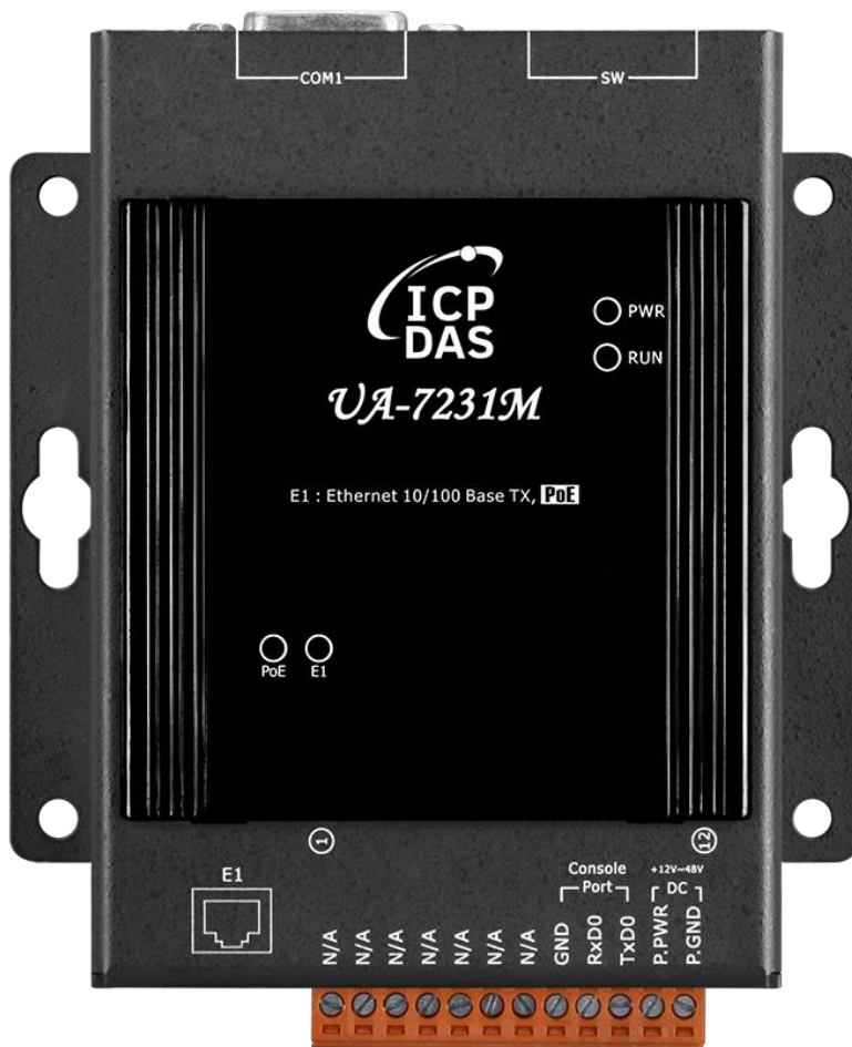
Fig. 282) UA-7231M LED Indicators
