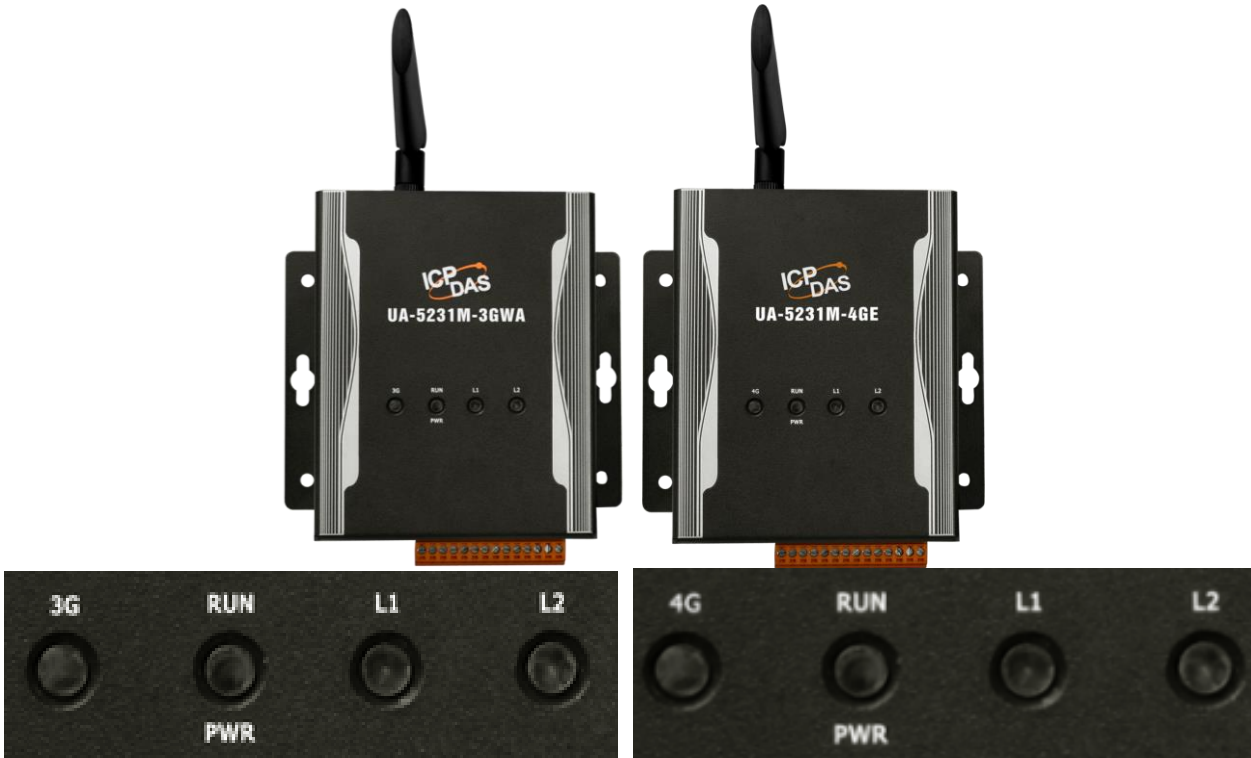
Fig. 280) UA-5231M-3GWA/-4GE/-4GC LED Indicators
