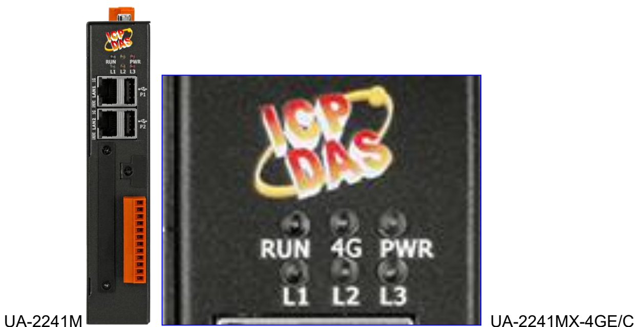
Fig. 281) UA-2241M/-4GE/-4GC LED Indicators
